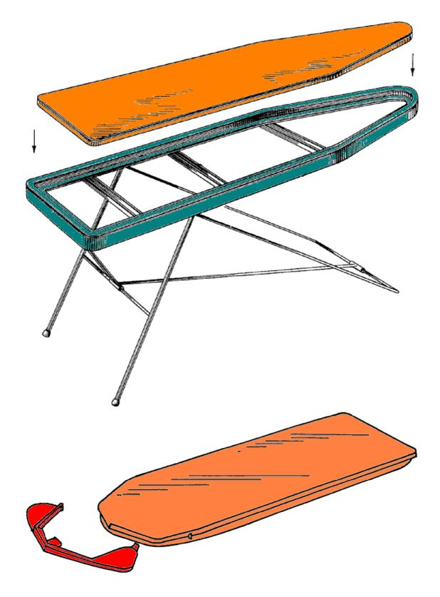
Sleeve boards; Attaching means therefor
