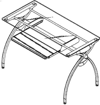
Figure 2. Example of a design for a workstation having tubular supports, transparent top, and shelf below work surface.
