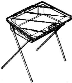
Figure 1. Example of a design for a workstation having tubular supports, transparent top, and shelf below work surface.
