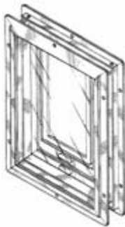
Figure 3. Example of a design for a two way pet door and frame.
