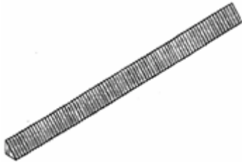
Figure 4. Example of a design for a weatherstrip.
