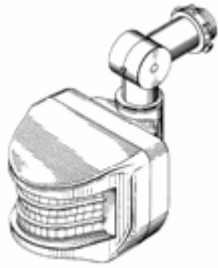
Figure 1. Example of a design for a motion or occupancy sensor that is part of a light fixture.
