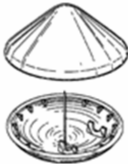
Figure 2. Example of a design for a pin-type antitheft alarm used on clothing.
